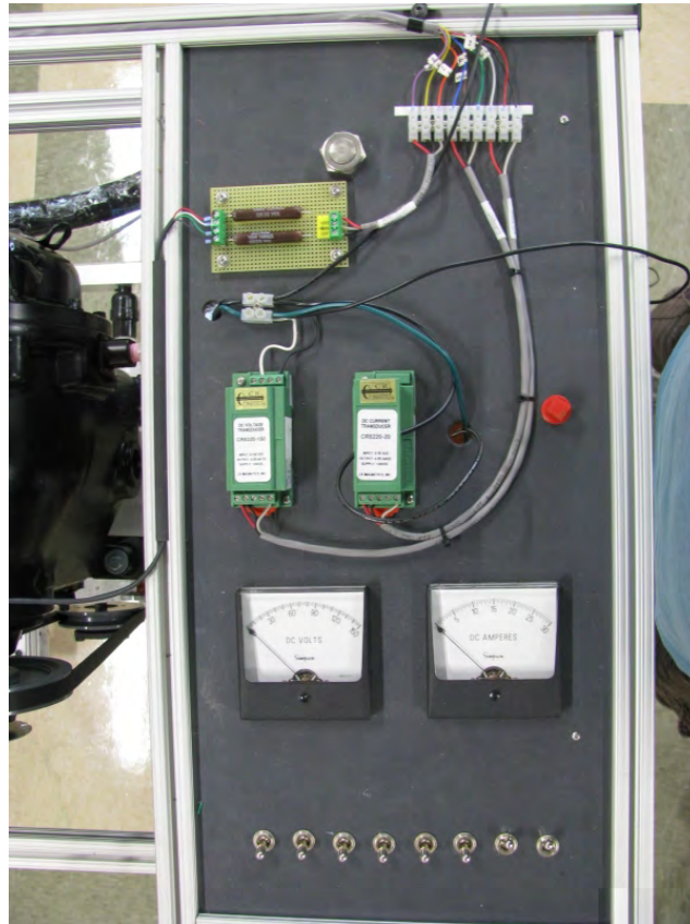
Figure C.5 Photograph of the voltage and current transducers
