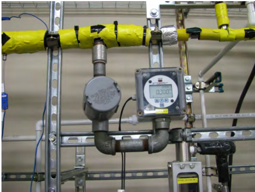
Figure C.7 Photograph of the vapor flow meter
