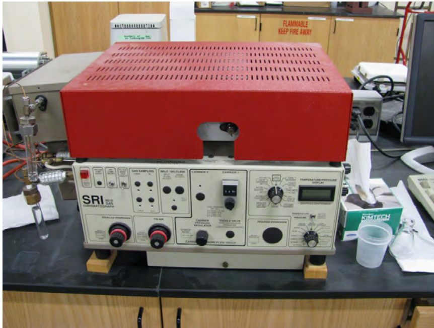
Figure C.1 Photograph of the gas chromatograph device used to calculate ammonia concentration
