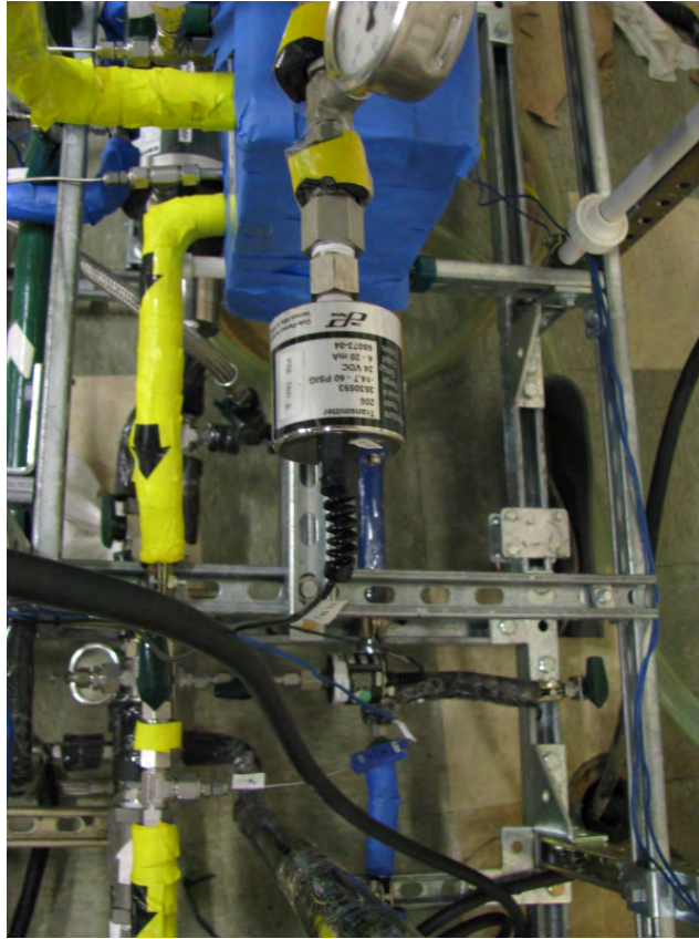
Figure C.4 Photograph of a pressure transducer
