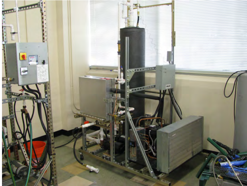
Figure 4.12 Photograph of the chiller used in the experiments
