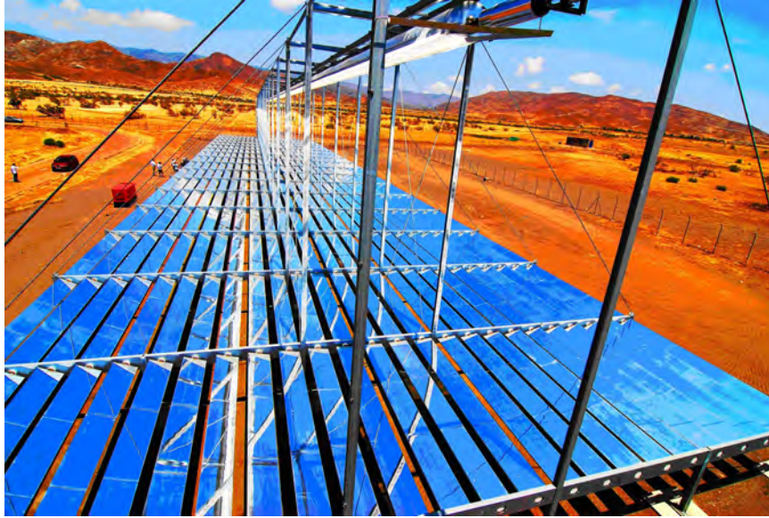
Figure 2.4 Solar power group's fresnel mirror test rig at the plataforma solar de Almeria in Spain. Photo is taken from [17]
